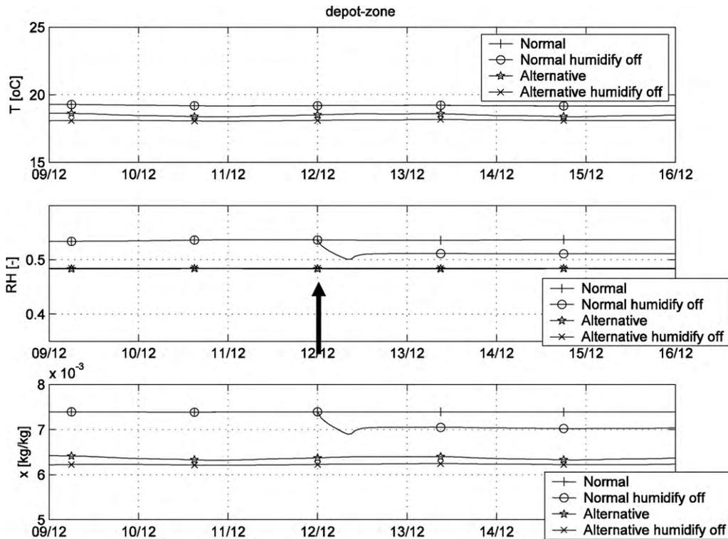
Fig. 11. Evaluation of humidification faults (arrow: time of failure).
