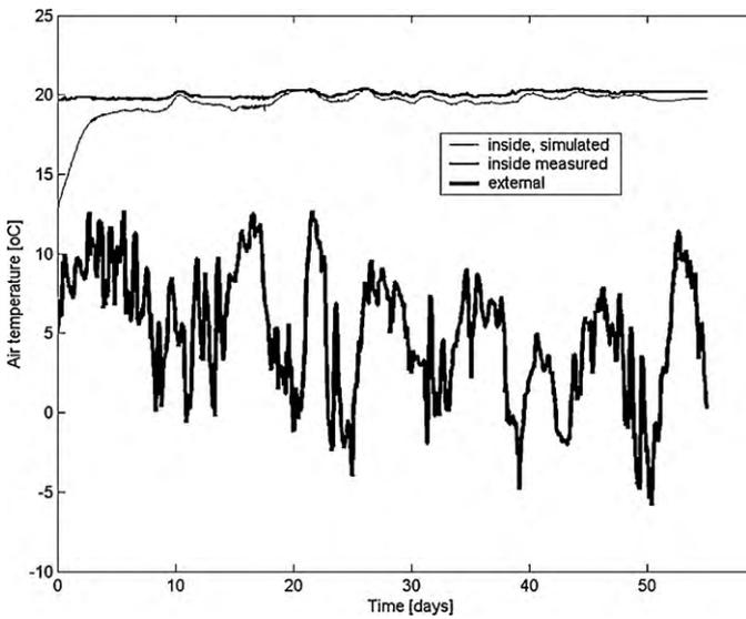
Fig. 7. Measured external and indoor air temperature and simulate indoor air temperature.
