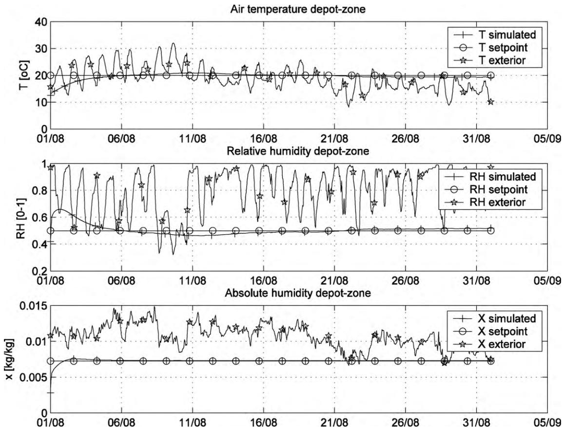
Fig. 9. The measured and simulated indoor climate in the depot.
