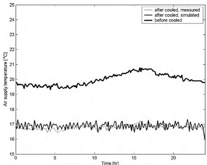
Fig. 6. Air temperature before and after the cooling coil.
