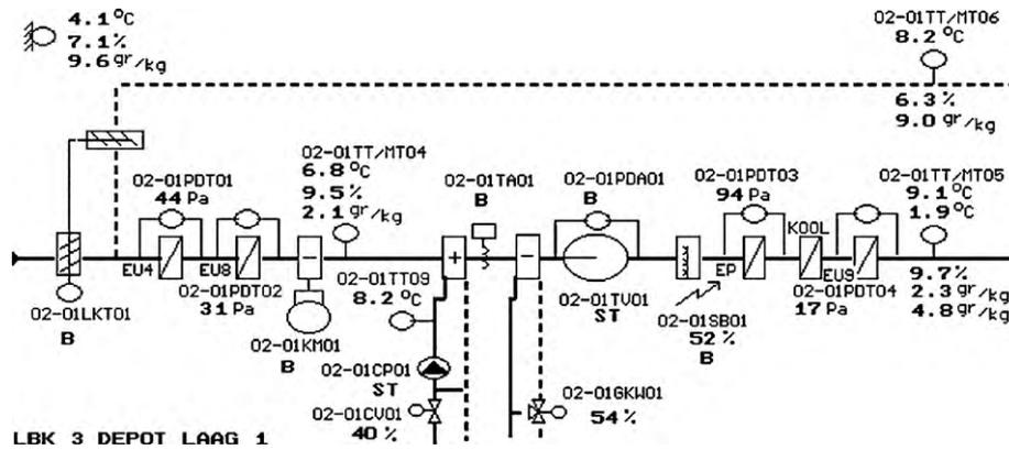
Fig. 5. Overview of the location and typical output of the sensors present in the system.
