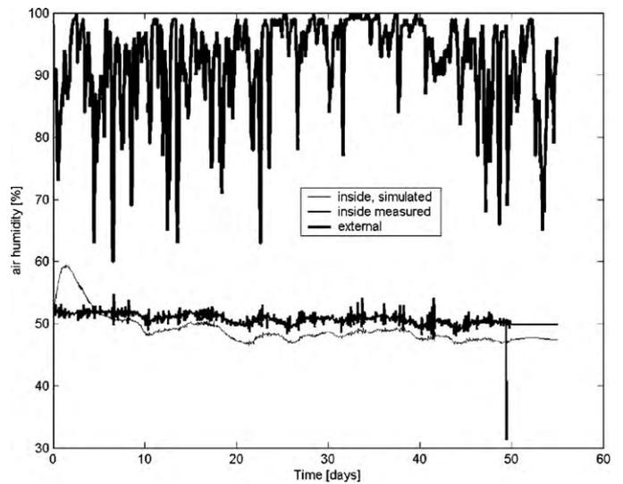
Fig. 8. Measured external and indoor relative humidity and simulate indoor relative humidity.
