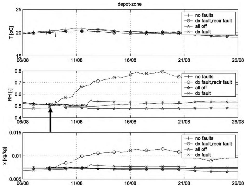
Fig. 10. Evaluation of dehumidification failures (arrow: time of failure).
